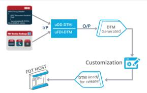
The device integration standards like EDDL, DTM and FDI allows consistent commissioning, configuration and maintenance of field devices. Based on the customer need, device suppliers need to provide and maintain EDDL, FDI Device Package and / or DTM. And in the entire Device Development Cycle, DTM will be the last piece in the puzzle and will always go through the tight schedule and budget constraint.
